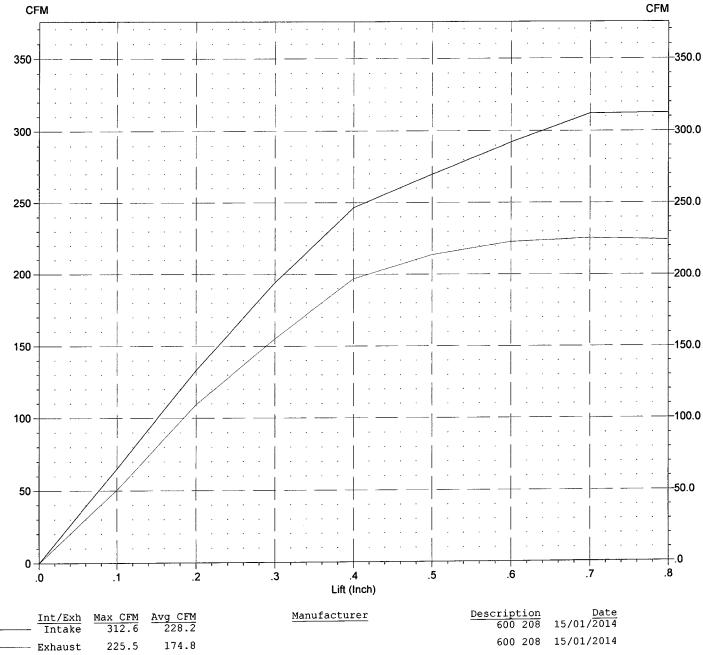
COME Racing Alloy VN 600 Series head. 2.08" intake and 1.60" exhausts. Test pressure 28" Intake flow Horsepower potential 0.500" = 556 HP and .643 HP 0.700" lift. Exhaust flow 0.10" = 135 cfm 0.700" lift. These are "out of the box" flows with only bowl blending by hand from the bottom of the seats and 1/4" down the bowl, a 30 second operation per bowl. These "600" heads have 207cc intake runner volumes.
